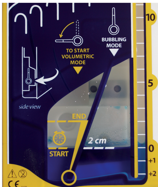
Fig. 1. The volumetric air leak meter contained within the chest drainage system that was used in the study. Air leaks are qualitatively assessed in the 'bubbling mode' and quantitatively graded in the 'volumetric mode' using the volume of water contained in the water-seal chamber (45 ml) as a unit of measure.
